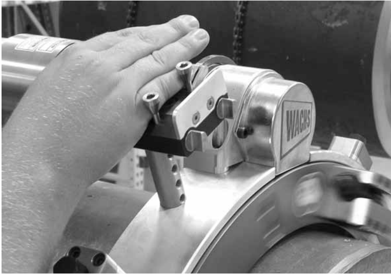
Figure 5-5. Push the trip knobs forward to engage the trips
