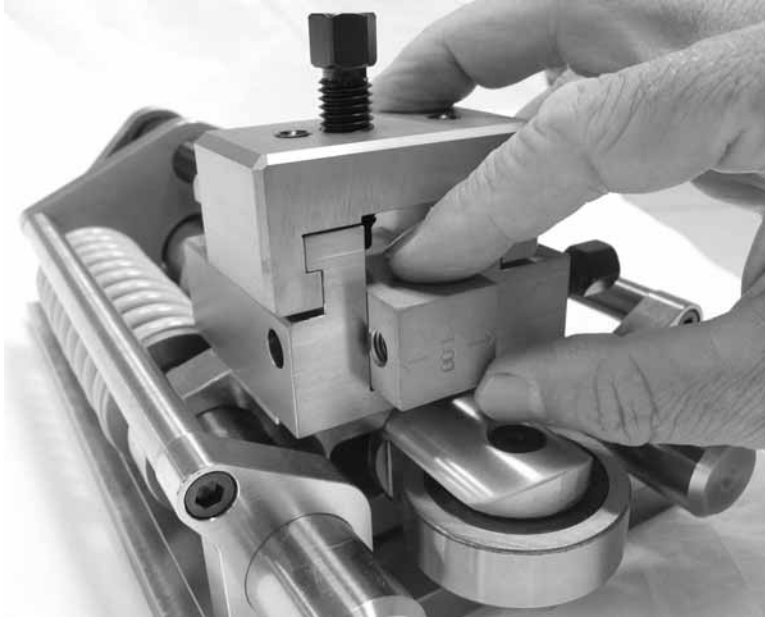
Figure 6-4. Insert the spacer into the tool block in the required orientation, with the threaded hole aligned with the screw hole.
