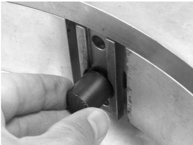
Figure 4-4. Press the clamp pad into the hole on the clamp leg or extension. The rubber o-ring holds the pad in place.
