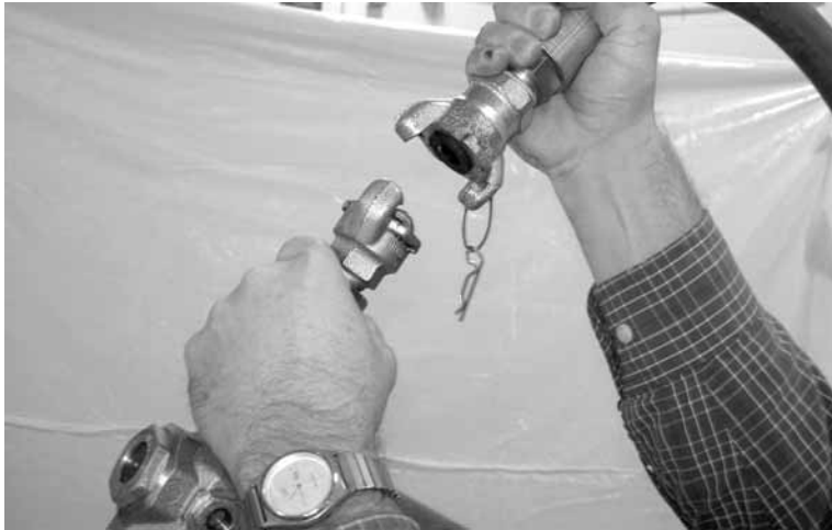
Figure 2-5. Disconnect pneumatic power by removing the air line from the pneumatic drive.
