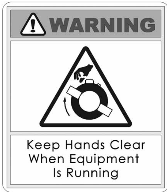
Figure 2-14. The “Keep Hands Clear” label is attached to the stationary ring of the MDSF. Stay clear of moving parts when the machine is operating. (Part no. 60-363-00.)
