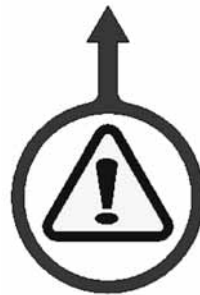
Figure 2-16. The alignment pin location label is attached to indicate the alignment pin holes. Two labels are on the MDSF, one for each pin location. (Part no. 60-1275-00.)
