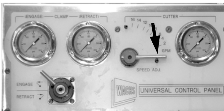
Figure 3-23. Set the cutting drive speed lever to 0 before starting the mill.
