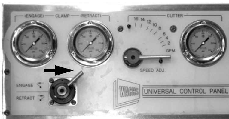
Figure 3-31. Set the clamping (auto-plunge) direction lever to the RETRACT position.
