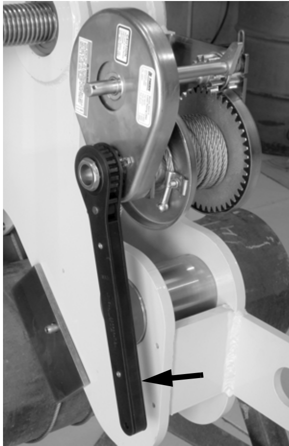
Figure 3-7. Push the ratchet handle forward to tighten the cable.
