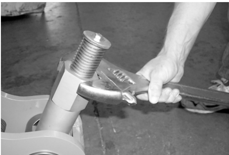
Figure 3-5. Tighten the chains to secure the rail mill to the workpiece.
