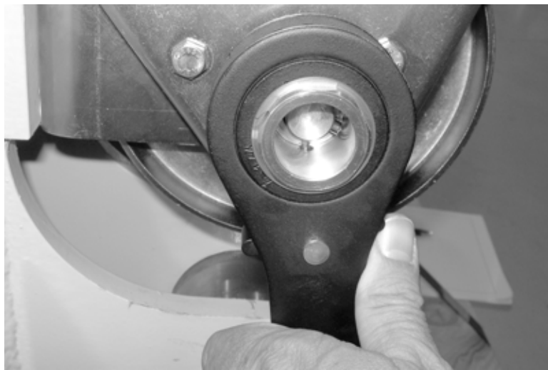
Figure 3-36. Push the right-side ratchet knob up to set the ratchet direction forward.
