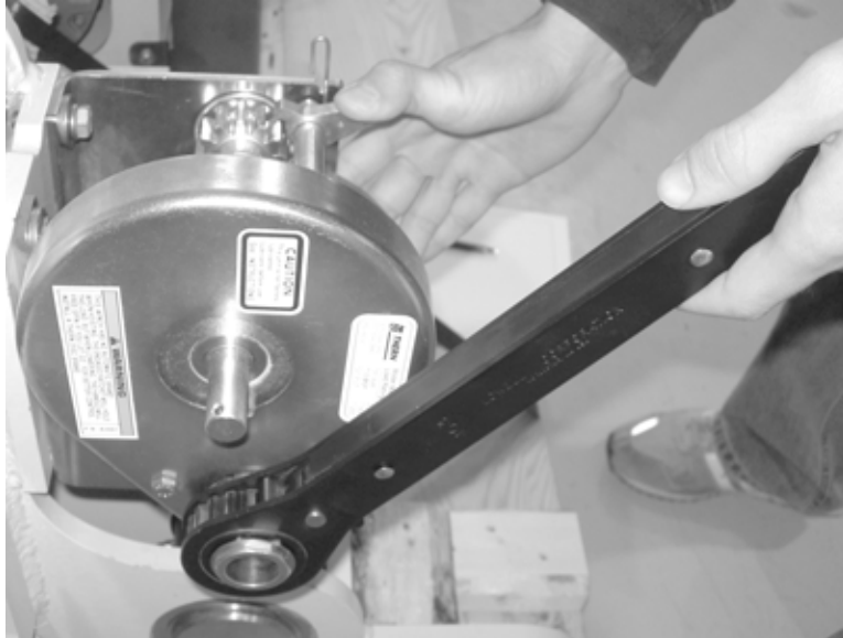
Figure 3-37. Turn the handle just enough to release the catch.
