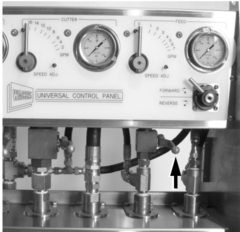
Figure 3-28. With the feed direction lever in the FORWARD position, move the feed drive lever up to start the drive. Then move the feed adjustment lever to start flow to the feed drive.
