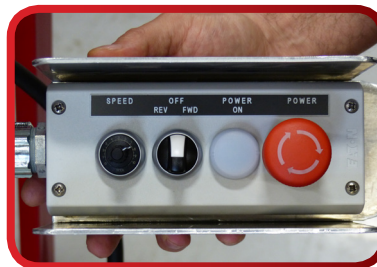
Standard remote control pendant includes flow direction, pump speed and E-stop
