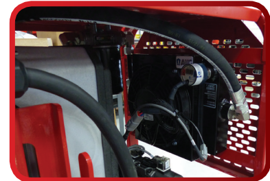
Heavy duty cooling and hydraulic manifold help keep fluid temperatures down
