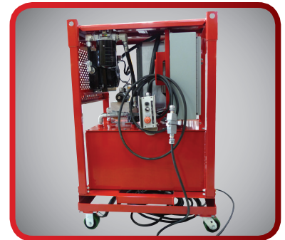
Steel cabinets are designed to protect power and control circuitry from damage
