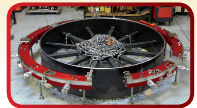
Four standard LDSF sizes cover a range of 60" to 120" (DN1500-3000) O.D. with a 15" (381mm) capacity between sizes
