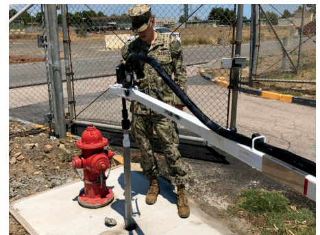
The extended reach ERV-750 valve exerciser allows valve operation from the roadside.
