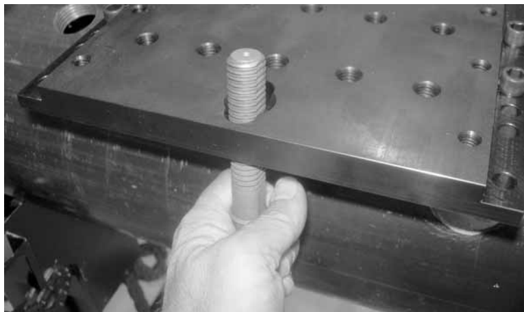
Figure 3-7. Insert the threaded end of the clamping chain through the hole in the saddle.
