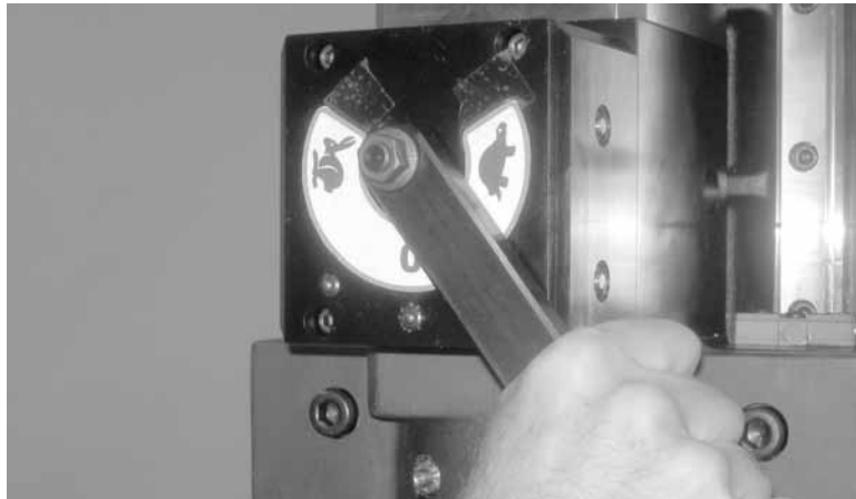
Figure 3-29. The photo shows the speed select lever in low speed mode.
