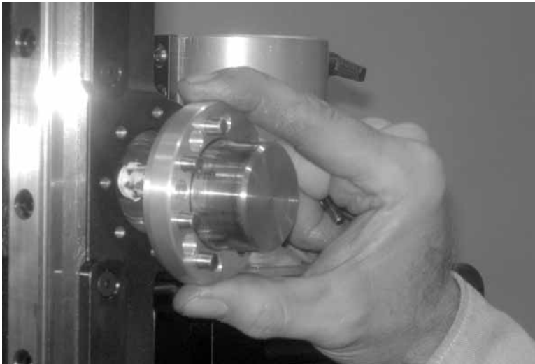
Figure 4-19. Put the feed lock housing on the other side of the drill, with the dowel pins toward the front of the drill.
