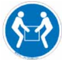
Figure 2-14. The two-person lift label is on both sides of the machine. Do not lift the machine by yourself. (Use of a lifting device is recommended.)
