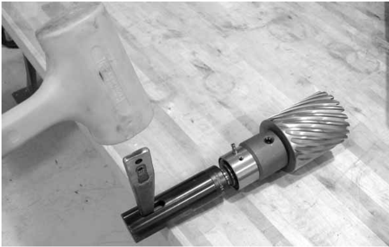
Figure 3-61. Use the drift to remove the chuck from the MT adapter. Tap the drift with a hammer if necessary.
