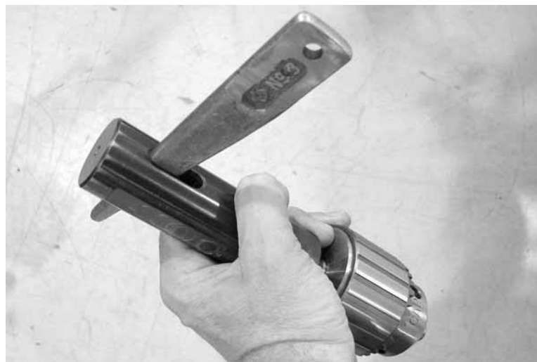
Figure 3-39. Use the drift to remove the chuck from the MT adapter. Tap the drift with a hammer if necessary.
