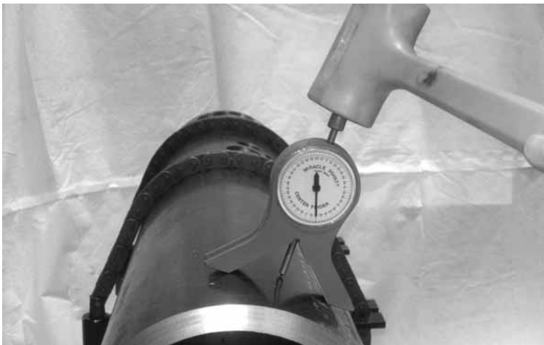
Figure 3-12. Using a mallet or hammer (not supplied), tap the punch to mark the hole location.
