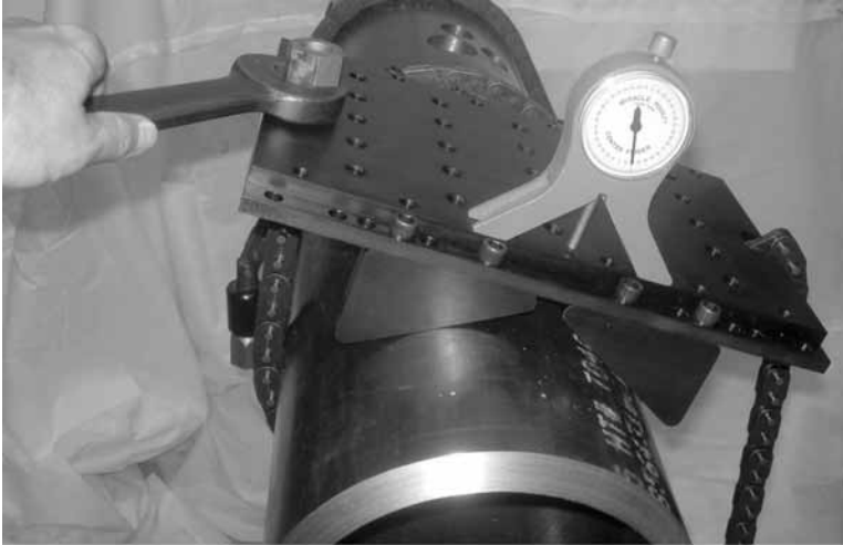
Figure 3-15. Tighten the chain tensioning nut with the saddle at the desired angle.
