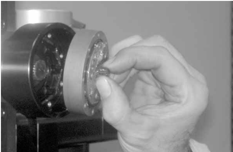
Figure 4-11. Pull out the feed reduction planetary gearbox.
