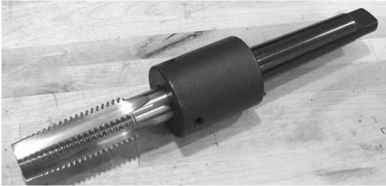
Figure 3-47. Assemble the tap and holder.
