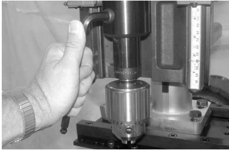
Figure 3-42. Tighten the spindle set screw.
