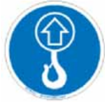
Figure 2-13. The lifting point label is on the frame in 2 places next to the lifting eyes. Always lift the machine using the lifting eyes. Do not lift on any other component.
