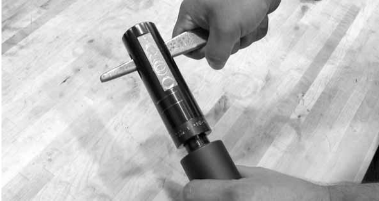
Figure 3-54. Use the drift to remove the chuck from the MT adapter. Tap the drift with a hammer if necessary.
