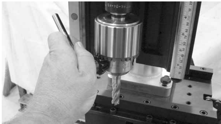
Figure 3-43. Insert the end mill in the chuck and tighten it using the chuck key.
