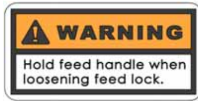
Figure 2-9. This label is on the feed lock clamp. Hold the feed lever when you loosen the feed lock lever. The spindle assembly could fall when loosening the lock, causing personal injury or equipment damage.
