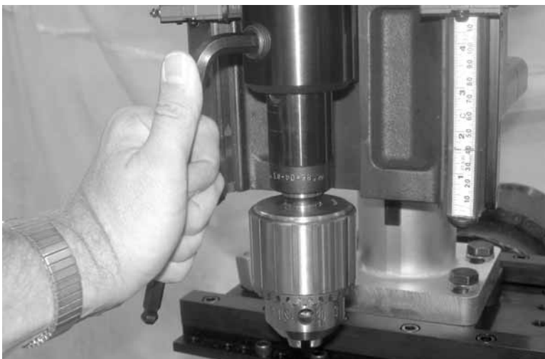
Figure 3-34. Tighten the spindle set screw.
