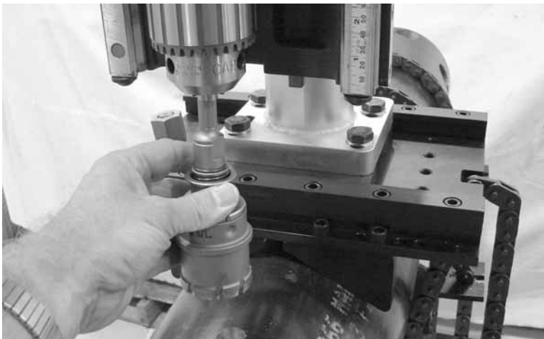
Figure 3-58. For chuck-mounted hole saws, insert the hole saw shaft into the chuck and tighten it using the chuck key.
