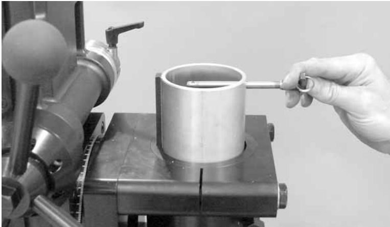
Figure 2-5. Insert the over-feed pin through the top of the support column before operating the drill.
