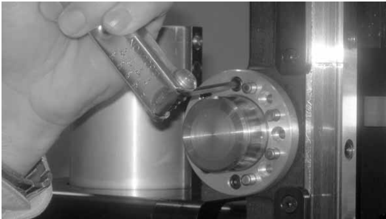
Figure 4-7. Remove the 5 screws around the back of the feed lock housing.
