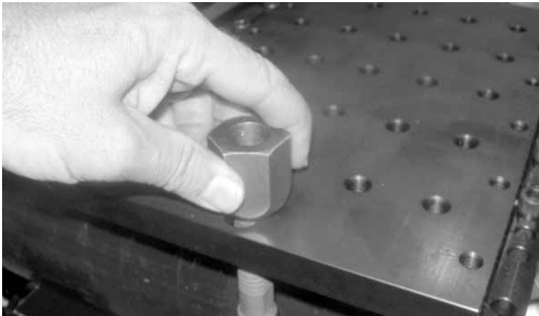
Figure 3-8. Install the chain tensioning nut on the threaded end of the chain.
