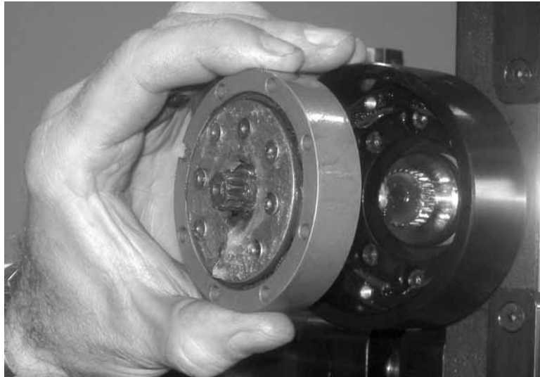
Figure 4-16. Replace the planetary gearbox in the feed reduction housing.
