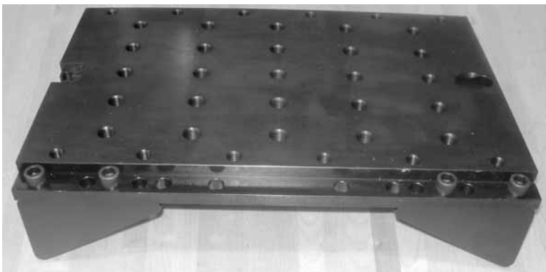
Figure 3-5. The photo shows the mounting shoes in the outer position, for pipes 22"-24" (558-610 mm) diameter.
