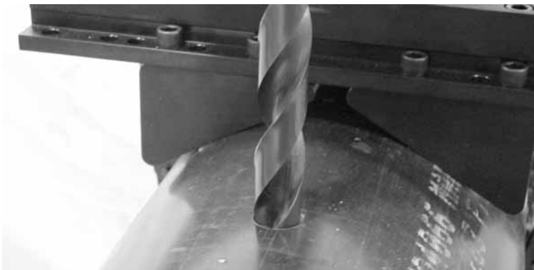
Figure 3-38. Feed the drill into the pipe.
