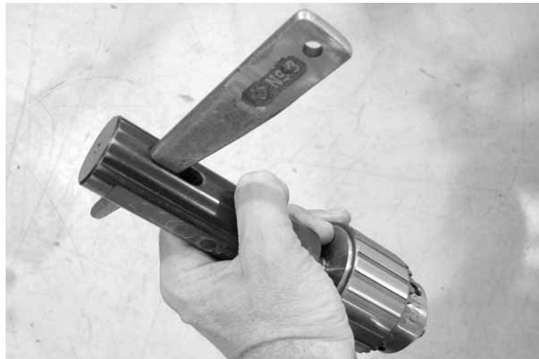
Figure 3-46. Use the drift to remove the chuck from the MT adapter. Tap the drift with a hammer if necessary.
