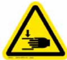
Figure 2-10. The crush injury label is on both sides of the PowerDrill. Support the machine with a lifting device when making any adjustments.
