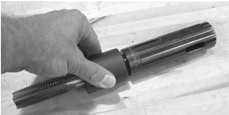
Figure 3-48. Insert the tap holder into the appropriate size MT adapter.
