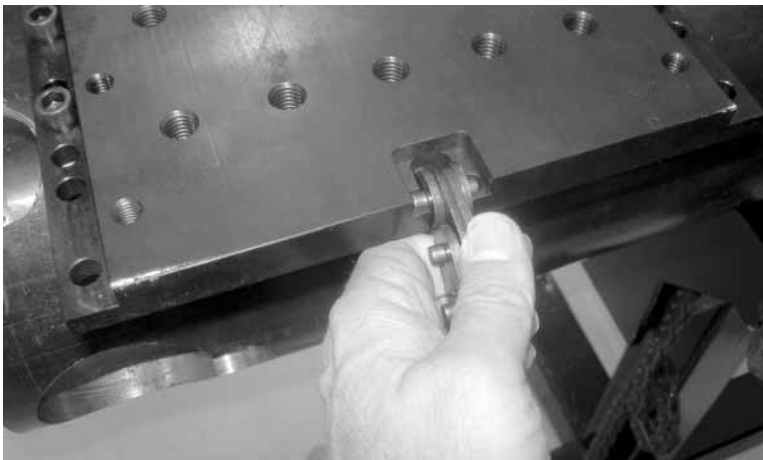
Figure 3-9. Pull the chain tight around the pipe and engage the closest cross pin in the slot.
