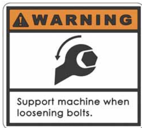
Figure 2-8. This label is on the axial column clamp on the back of the drill. Make sure to support the drill on the column when loosening the height adjustment bolts. The drill could slide down the column, causing personal injury or equipment damage.
