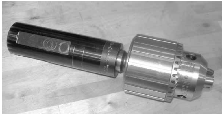
Figure 3-31. Insert the chuck into the MT #3 adapter.
