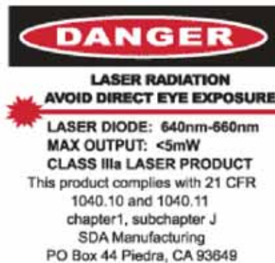
Figure 2-15. The laser exposure label is on the optional laser center. Avoid eye exposure with the laser.
