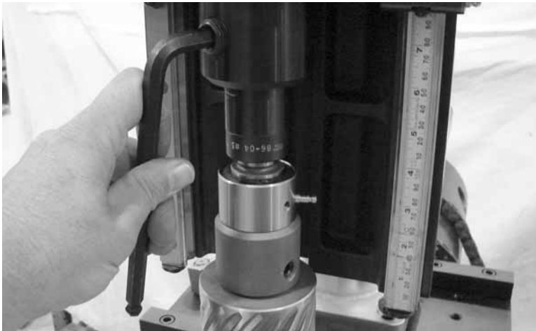
Figure 3-57. Tighten the spindle set screw.
