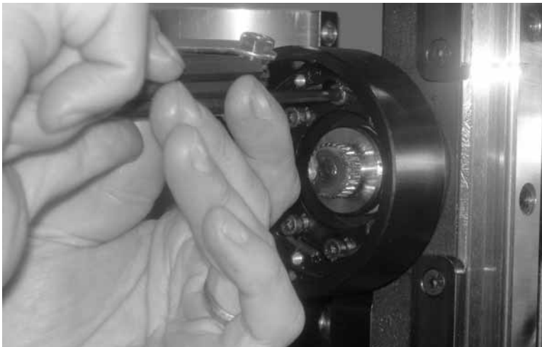
Figure 4-15. Insert the screws into the feed reduction housing.
