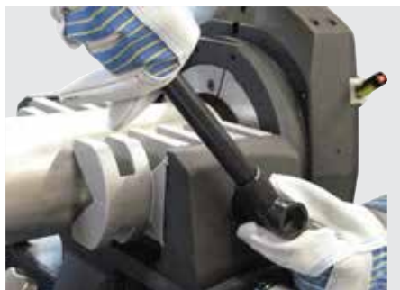
Fixture for clamping jaws (GF 4 (AVM/MVM) only)
