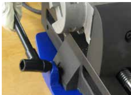
Fixture of the saw for quick-mounting plate
