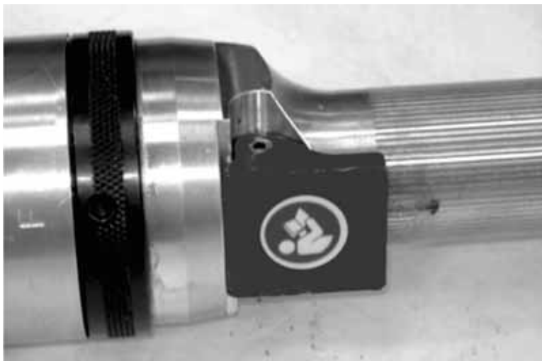
Figure 5-93. The photo shows the correct installation of the open throttle plate.
