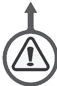
Figure 2-21. The alignment pin location label is attached to indicate the alignment pin holes. Two labels are on the LCSF, one for each pin location. (Part no. 60-1275-00.)
