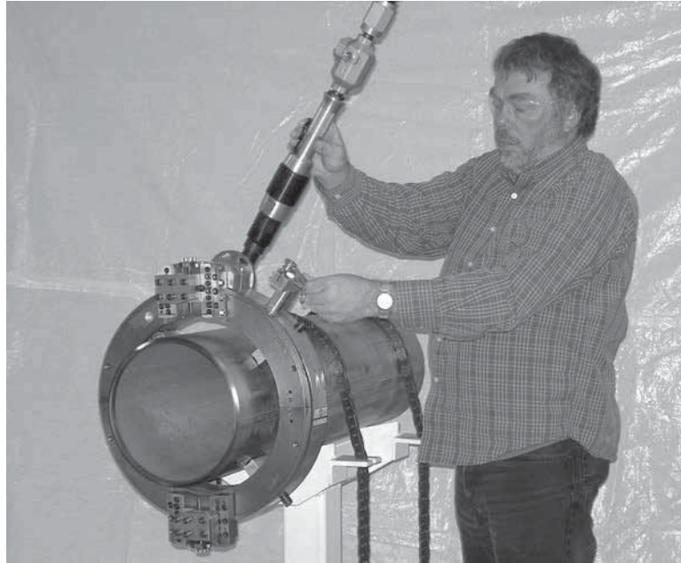
Figure 2-7. If possible, stand behind the LCSF to stay clear of moving parts while operating the controls.
