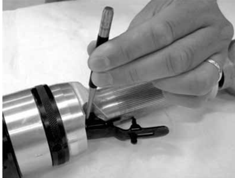
Figure 5-90. Use a punch to drive out the pin holding the air trigger.
