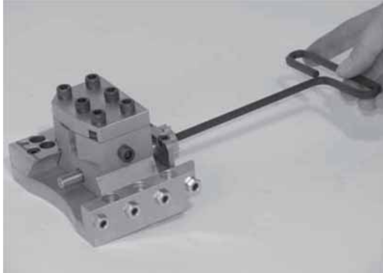
Figure 7-30. Check the tension on the slide by driving it to both ends of the feed screw.
