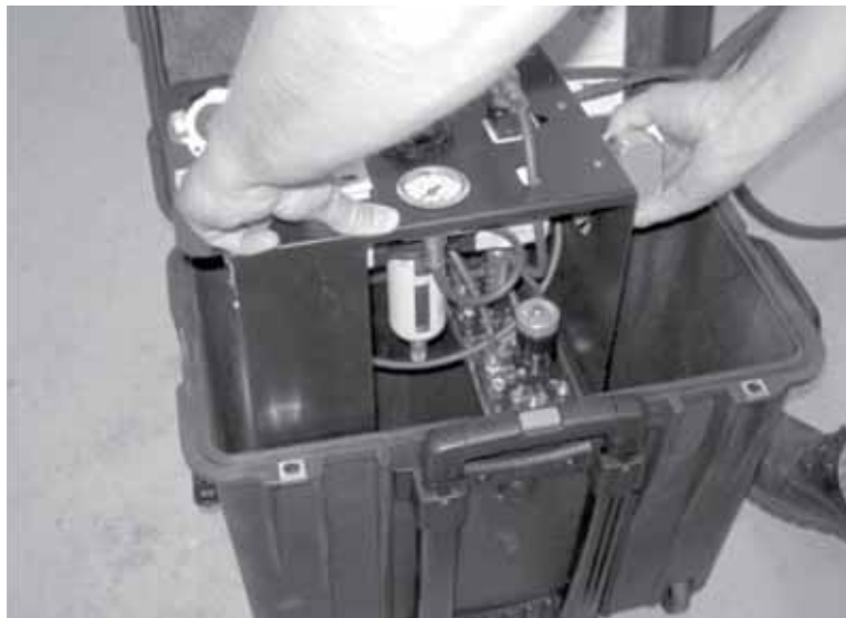
Figure 6-8. Lift the control panel out of the case for service or to drain out accumulated water.
