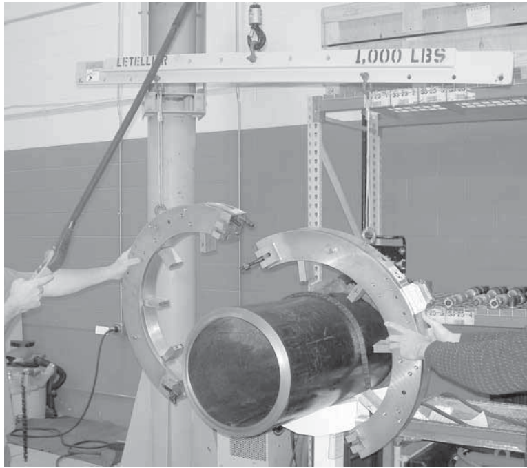
Figure 5-12. Assemble the ring halves around the pipe as shown.
