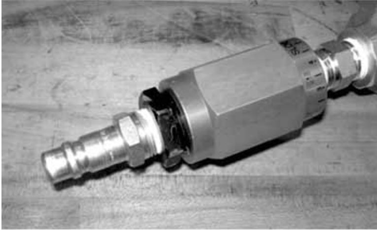
Figure 5-89. Install the supplied nipple onto the air motor for use with the ACM.
