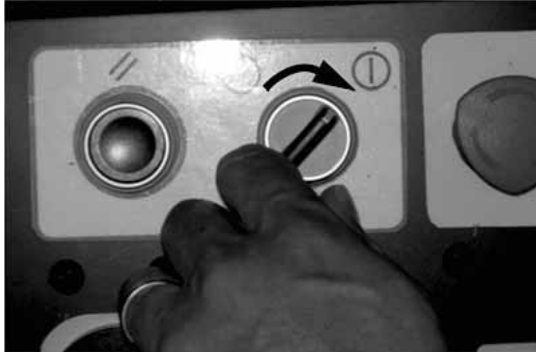
Figure 5-82. Turn the Remote Enable switch on to allow operation using the handheld pendant.
