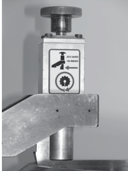
Figure 5-69. Axial (.0312) and radial (.0784) adjustment per revolution
