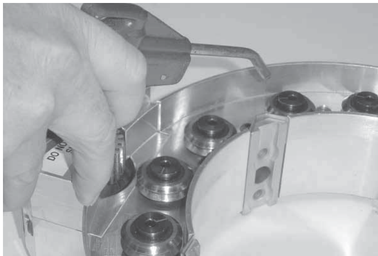
Figure 7-12. Clean debris from the stationary ring.
