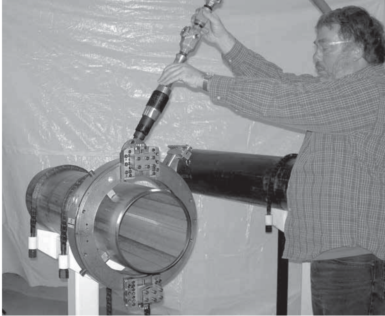
Figure 2-8. When operating the LCSF from the front, stand to the side of the machine to operate the controls without reaching across the rotating ring.
