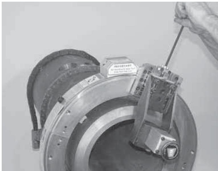
Figure 5-68. Adjust the counterbore slide by turning the radial feed screw clockwise
