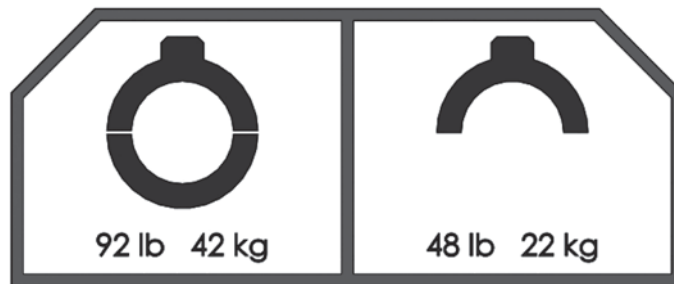
Figure 2-18. Weight labels for the LCSF are attached to the pinion housing. Weights and part no. vary according to LCSF model. (Part no. 60-1279-XX.)
