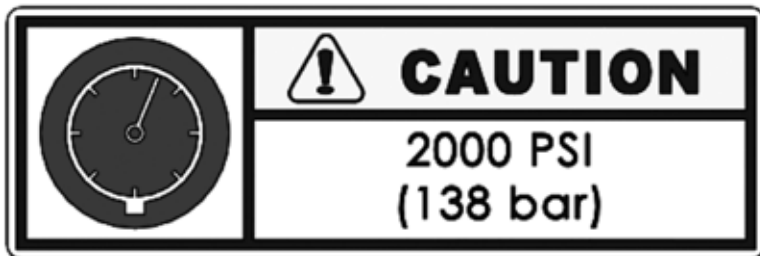
Figure 2-5. The hydraulic pressure limit label is on the hydraulic motor. (Part number 90-402-01.)
