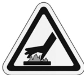
Figure 2-6. The hot surface warning label is on the hydraulic drive. (Part number 90-403-00.)
