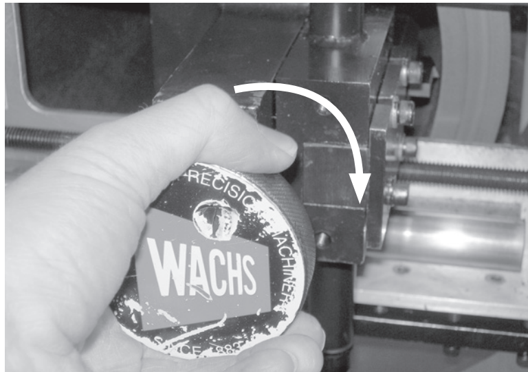
Figure 3-29. Retract the male tool slide using the feed knob.
