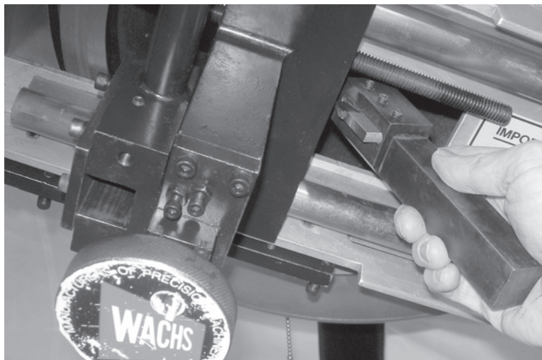
Figure 3-9. To install the tool holder, you can reach through the slide and insert the holder into the front of the tool block.
