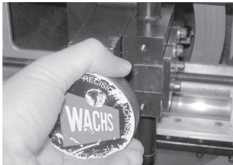
Figure 3-21. Retract the tool out of the pipe by turning the feed knob clockwise.
