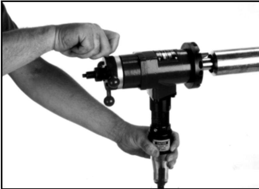
Wachs **SDB 103/3**, a hand held beveling machine that delivers maximum power and performance for fast, accurate weld preps on pipe and tube from 1.16" I.D. thru 4.5" O.D. (28 mm to 114.3 mm)
