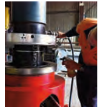
ECC can be used inverted for cut lines close to the flange
