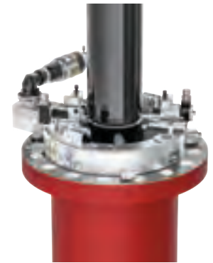
Simultaneously cuts and bevels casing
