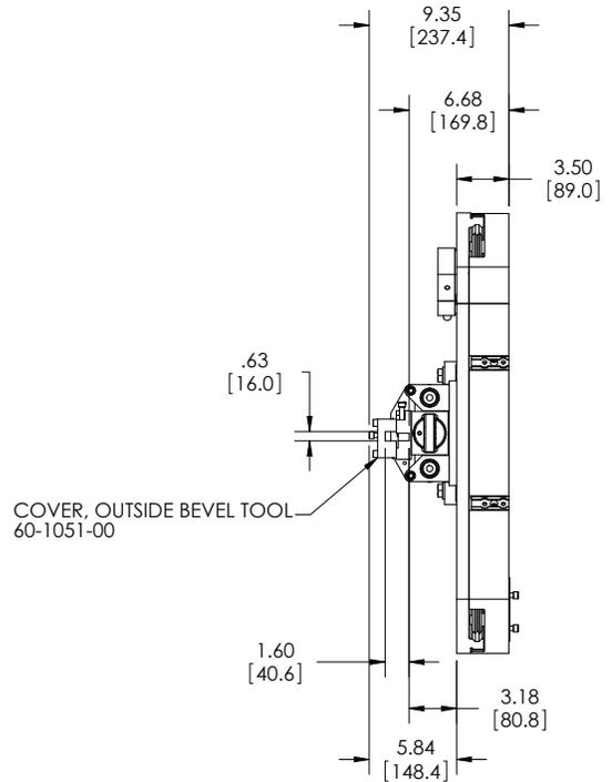
DIMENSIONS IN BRACKETS ARE MILLIMETERS
