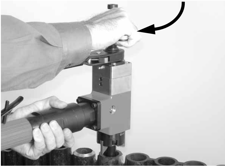
Figure 5-27. Turn the clamp handle to tighten the clamp legs in the tube.
