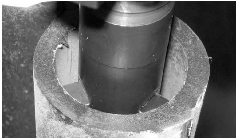
Figure 5-25. Hold the MB Plus in place with the legs 1/2"-3/4" (12-19 mm) inside the tube end.
