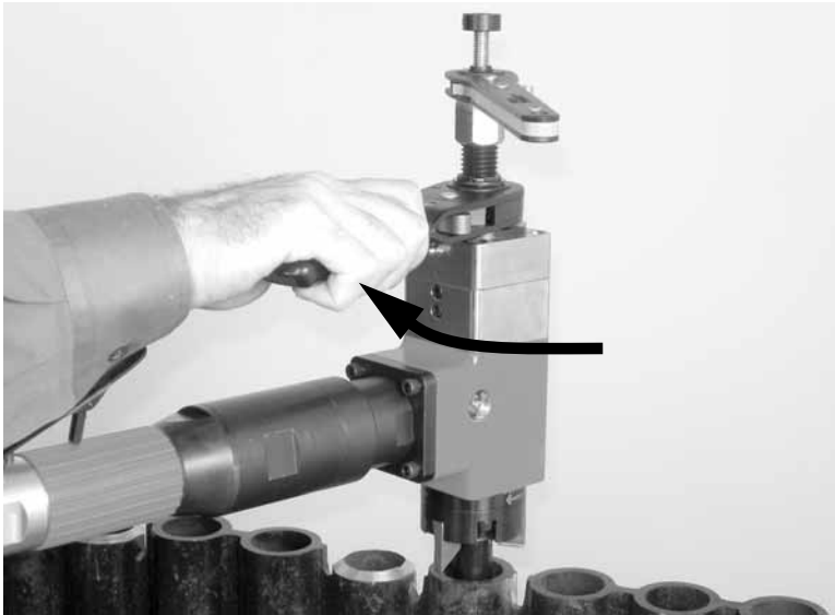
Figure 5-33. Feed the tool head into the workpiece using the feed handle.
