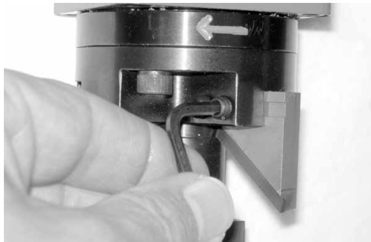
Figure 5-23. Tighten both set screws to secure the tool.
