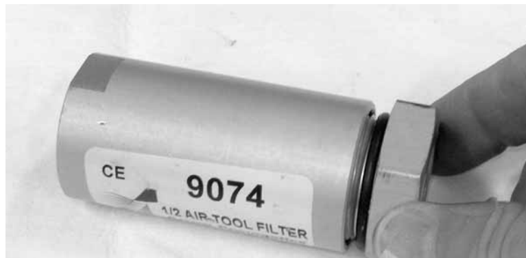
Figure 6-11. Replace the end cap on the filter cartridge and snug it with a wrench.
