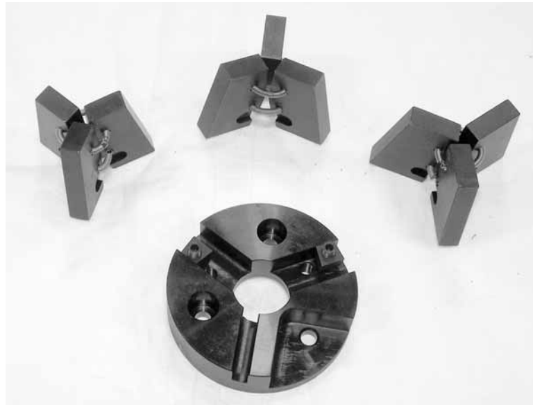
Figure 3-5. An optional extender kit includes a larger tool head and 3 leg sets for I.D. up to 3.0" (76.2 mm) and O.D. up to 3.25" (82.6 mm).
