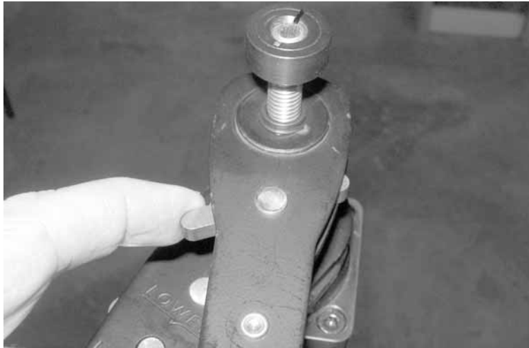
Figure 5-35. Set the knob on the clamp handle to the release direction.
