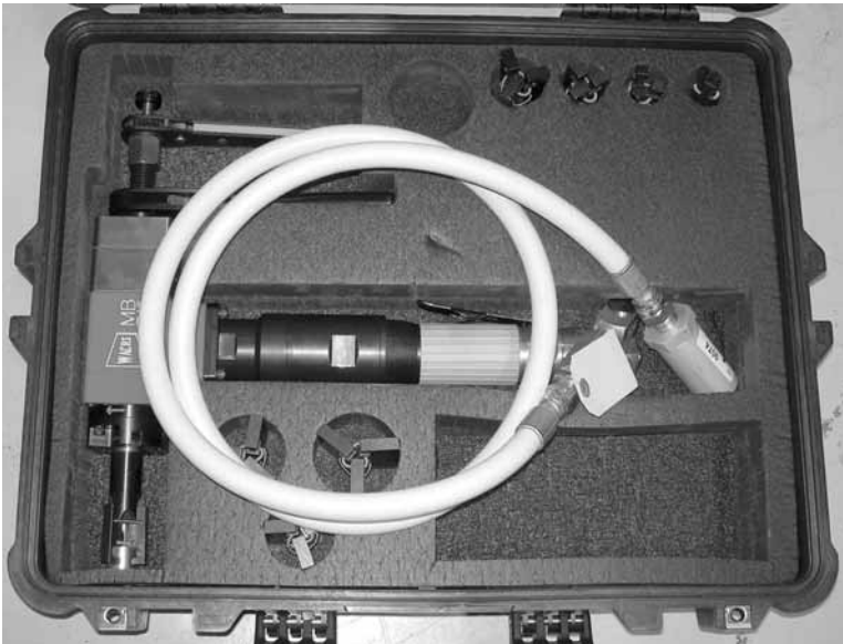
Figure 4-1. Store the MB Plus and its accessories in the case provided. Compartments are provided for all standard and optional components.
