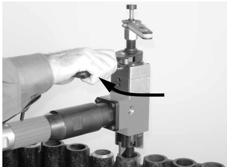
Figure 5-29. Turn the feed handle clockwise to feed the tool head.
