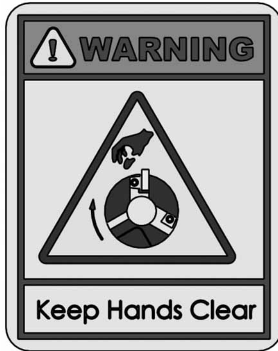
Figure 2-1. This Warning label (part number 71-062-00) is on the MB Plus machine.
