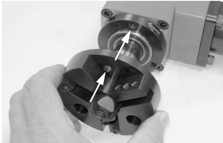
Figure 5-16. Slide the large tool head onto the mandrel. Line up the holes in the tool head and the main shaft.
