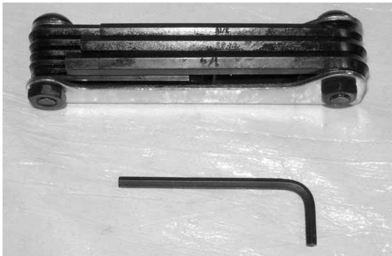
Figure 3-7. A hex wrench cluster and 1/8" short-arm hex wrench are provided for operation and maintenance of the MB Plus.
