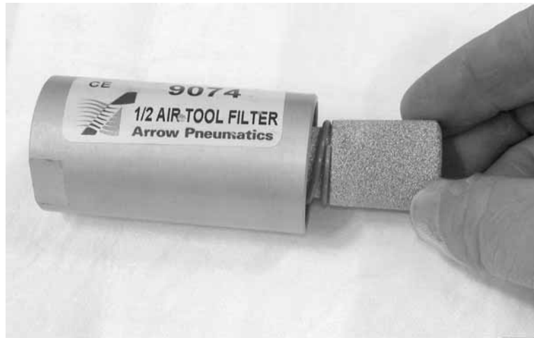
Figure 6-10. Replace the element in the filter.
