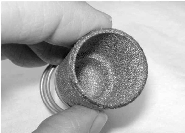
Figure 6-9. Inspect the inside of the filter element. (The photo shows an element in good condition.)
