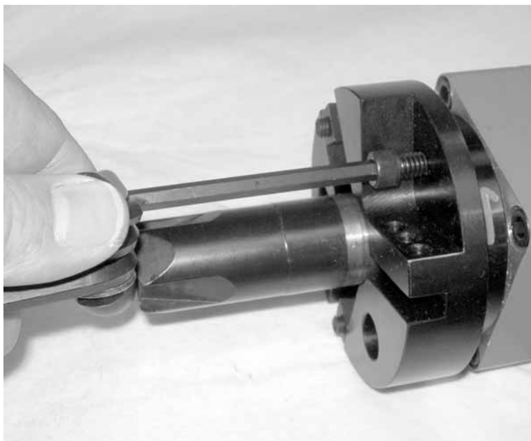
Figure 5-17. Install and tighten the 3 screws holding the tool head.
