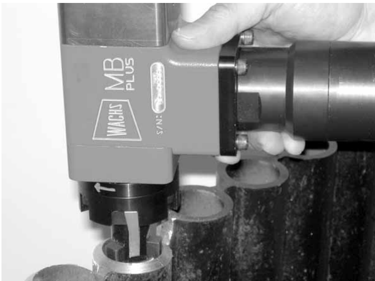
Figure 5-37. Pull the mandrel out of the tube to remove the machine.
