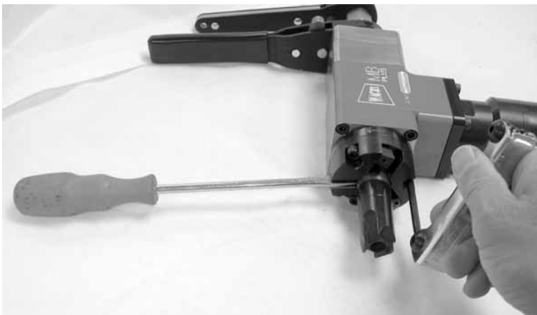
Figure 5-14. To keep the tool head from turning while loosening the screws, you can insert a screwdriver in the straight shank tool slot.
