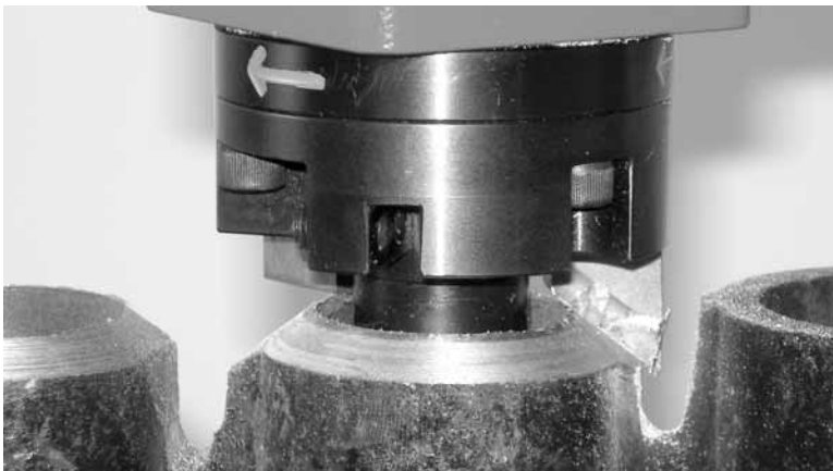
Figure 5-34. Apply continuous feed pressure for a smooth surface.
