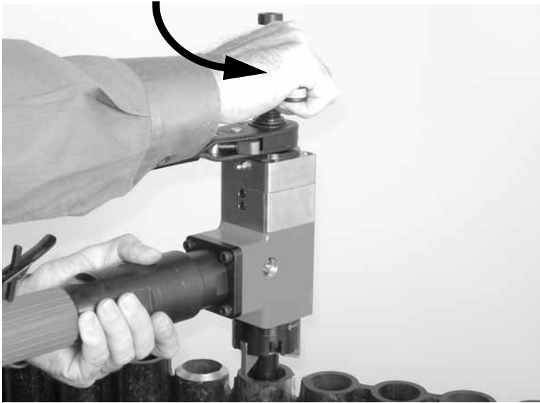
Figure 5-36. The clamp handle will engage counter-clockwise to loosen the legs in the tube.
