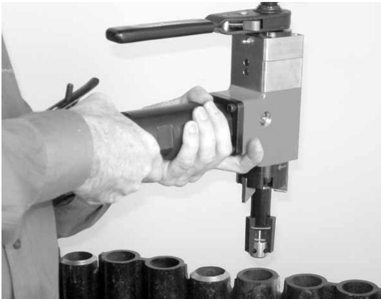
Figure 5-24. Insert the clamp legs into the end of the tube or pipe.
