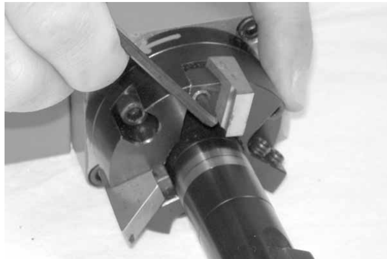
Figure 5-19. Tighten the wedge screw to secure the tool.
