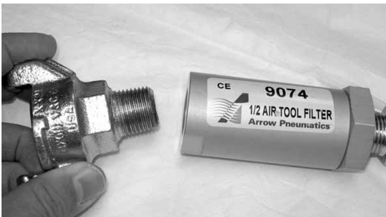
Figure 6-5. Remove any air line adapter from the filter.
