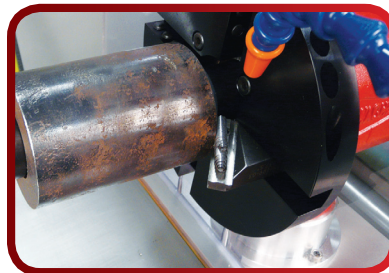
Wachs Coupon Station quickly puts the perfect weld bevel on your cut sections. Machining is visible through the enclosure
