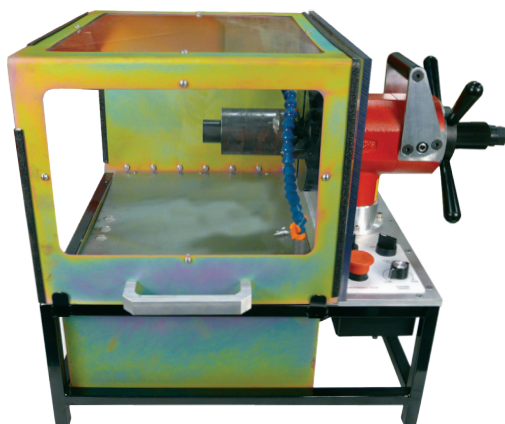
Wachs Coupon Station quickly puts the perfect weld bevel on your cut sections. Machining is visible through the enclosure
