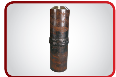
Welded coupon - to reuse simply cut out the old weld with your saw, re-prepare with the Coupon Station and weld again
